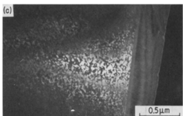
Figure 4 Air-cooled sample: (a) electron diffraction pattern; (b) dark-field image taken using (1 0 0) superlattice spot; (c) dark-field image taken using (\frac{3}{2} \frac{1}{2} \frac{1}{2}) superlattice spot.
